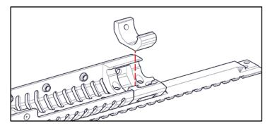
3. <u>Carefully</u> seat barreled receiver onto handguard. This is best done by rocking it into position as shown.
