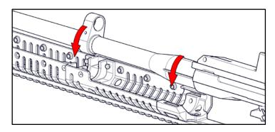
4. Install mounting hardware, starting with Modified Screw on Rear Mounting Block. Thread Modified Screw and Rear Block Screw into the Nut Plate. Note that you'll want to leave the Flanged Bolt & Clamp Screws hand tight in order to properly align top rail.
