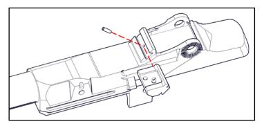
2. Install Barrel Clamp, orient as shown.
