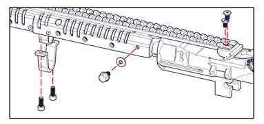
5. Align Upper Handguard to sights. Once straight, tighten Flanged Bolt & Clamp Screws. For best results, tighten Clamp Screws in alternating pattern.
