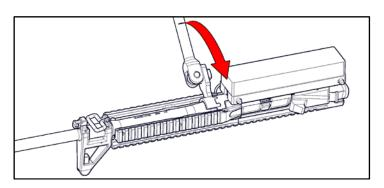
4. Use two included bolts to secure M203 Mounting Bracket to Receiver.
