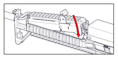
6. Once fully seated, use moderate thumb pressure to close locking tabs and secure lower handguard.
