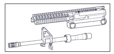
2. Lubricate barrel extension and gently install into receiver, insuring that the indexing pin of barrel extension is aligned with notch in VIS receiver.
