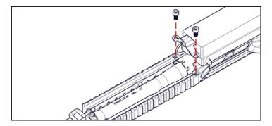
5. Install lower handguard, front first, into VIS receiver.
