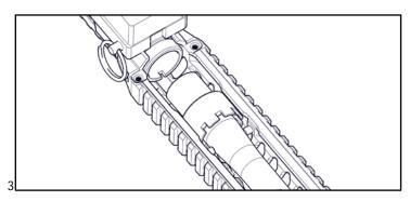
Apply anti-seize to threads of receiver and install Barrel Nut by hand.
