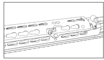
Once fully seated use moderate thumb pressure to close locking tabs and secure lower handguard.
