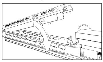
5. Install lower handguard, front first, into VIS receiver.
