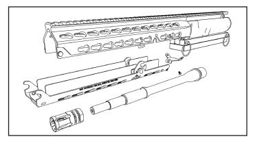
1. Install barrel nut onto barrel and secure VIS receiver on action block.
