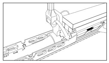
3. Apply anti-seize to threads of recevier and install barrel nut by hand. Once theaded, use the included barrel nut wrench to tighten barrel nut to 40 foot pounds (54.23 nm).
