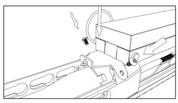
4. Use two included bolts to secure M203 mounting bracket to receiver.
