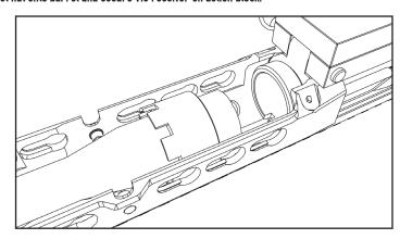
Lubricate barrel extension and gently install into receiver, ensuring that the indexing pin extension is aligned with notch in VIS receiver.
